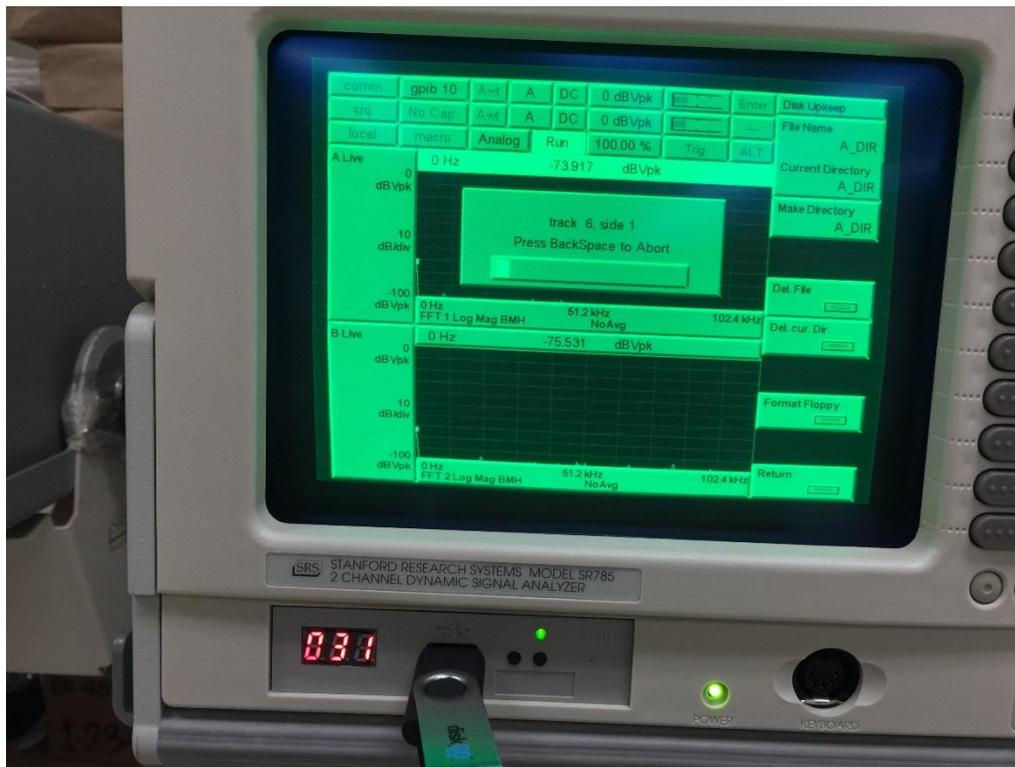
The SR780/SR785 can now retrieve data and settings from drive 000 (if the drive is set to 000) and it can retrieve data from drive 031 (if the drive is set to 031).
