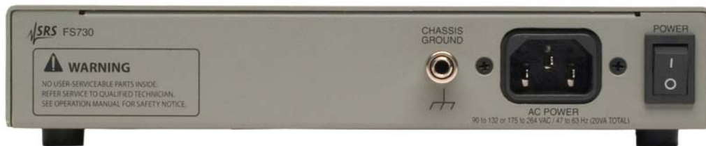
Figure 2. Rear panel of FS730 Distribution amplifier.
