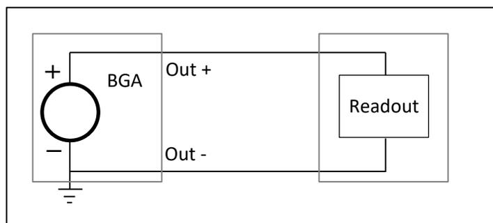
FIGURE 5: VOLTAGE OUTPUT
