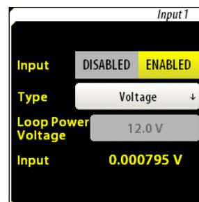
Certain pressure transducers can operate using loop power provided by the BGA244. This is the simplest type of transducer to integrate since it only requires 2 wires. See *Analog Inputs* (page 81) for details on different input types. If Current with Loop Power is selected, enter the appropriate loop power supply voltage.
