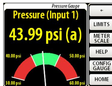
The Pressure Gauges each have a meter scale and limits similar to the Home page displays. Press [METER SCALE] to set the graph scale and [LIMITS] to set the Pressure Limit values. These are the over and under pressure limit values used on the Event Relay page.
