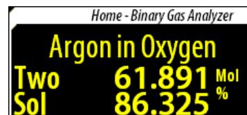
If a dual concentration is detected, the BGA244 reports both ratios. Concentration 1 is the smaller value and is displayed on top. Concentration 2 is the larger value and is displayed on the bottom.
