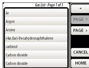
Select the desired gas by pressing its entry. This will enter the selected gas and return to the Select Gases page. If you wish to change the gas, press the desired gas selection key and re-enter the gas.
