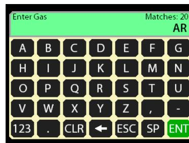
When the number of matches is down to a manageable number (< 20 or so), press [ENT] or [ENTER]. This will open up a list of all of the matches from the gas table. Note that matches can occur at any position in the gas name, formula or CAS #. If there are more than 7 matches, use [Page ↑] and [Page ↓] to view the entire list. If you don't see the expected gas, press [←] to return to the alphanumeric entry window.
