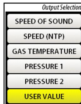
If User Value is selected, a User Setting entry box will appear below “Linked to”. Enter a value within the full scale range for that output type. Otherwise enter the Scale Min and Scale Max values for the linked parameter.
