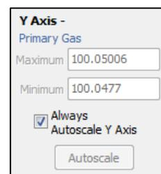
**[Autoscale Now]** scales the minimum and maximum values at the moment it was pressed.  **Always Autoscale Y Axis** will automatically rescale the display for each value acquired.
