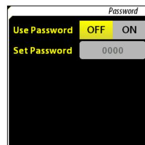
If you forget the password, the unit can be reset using Hard Reset function described in the *Hardware Reset* section. This will disable password locking and reset the password to the default value of 0000.
