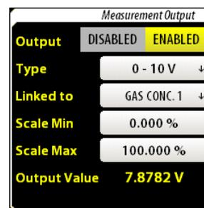
The present Output Value (voltage or current) is displayed just below Scale Max.
