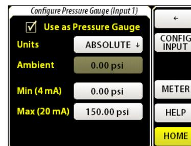
Assuming the formats match, enter the pressure values for the minimum and maximum analog input values. If the analog output of your pressure gauge doesn't match the span of the analog input, calculate what the pressure would be at those points.
