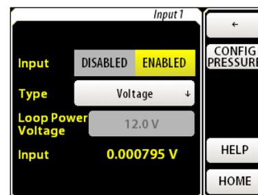
Analog inputs can be used as either general purpose inputs, or together with a transducer as a pressure meter. If an analog input is configured as a pressure meter it may not be used for general purpose measurements. In either case the input must be configured properly for the desired measurement. The Input reading displayed on this page is in V or mA regardless if the analog input is used as a pressure meter.
