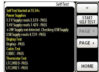
To begin Self Test, press [START SELF TEST]. The tests and their results will be written to the screen. Upon completion, the BGA244 will display “SELF TEST PASS” or “SELF TEST FAIL”. Use [PAGE↑] and [PAGE↓] to navigate the list of tests. If Self Test fails it will be listed on the Faults page.
