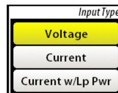
An improperly configured analog input, broken pressure transducer or wiring can lead to out of range pressure readings. If this occurs, a “BAD PRESSURE” screen message will appear in place of the measurement and no results will be reported. There are also several alerts that can occur for the analog inputs. These normally indicate a problem with the device connected to the Analog Input or wiring, rather than the input itself. See *Analog Inputs* (page 81) for details.
