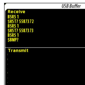
that interface. They can be helpful when debugging communication problems. Press the [BUFFER] key on the interface page of interest to view.
