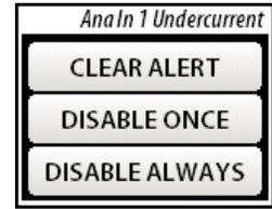
Press [DISABLE ONCE] to ignore a currently active alert. This will cause the alert to be ignored and clear the alert indicators (assuming this is the only active alert). The Alert button will turn lite grey to indicate its “disabled once” state. If this alert is cleared and later re-asserted, it will revert to the normal “un-ignored” state, with the alert indicators active.
