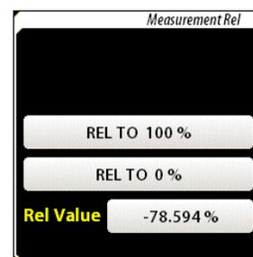
Press [REL TO 0%] to set the measured value to 0% (or 0 ppm or 0.0 fraction). The value required to force the displayed value to 0% is displayed in the [Rel Value] button in global ratio units.
