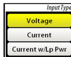
The Loop Power Voltage can be entered if Current w/Loop Power is selected. This can vary from 6 and 19 V. See *Analog Input* (page 27) for details on devices that can use loop power.
