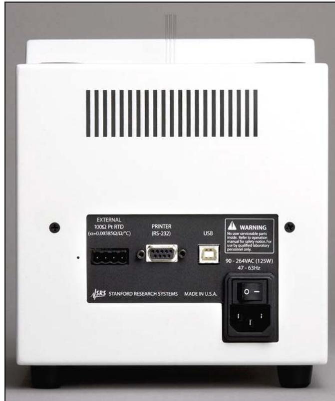
Figure 2. Back Panel of OptiMelt.
