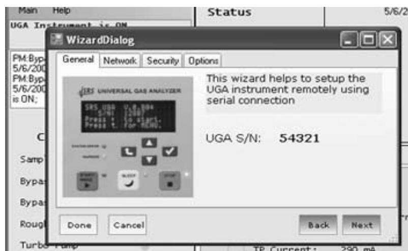
Fig. 2-4. Screenshot of the ‘Wizard’ dialog box in the Main menu of UGA control software.
