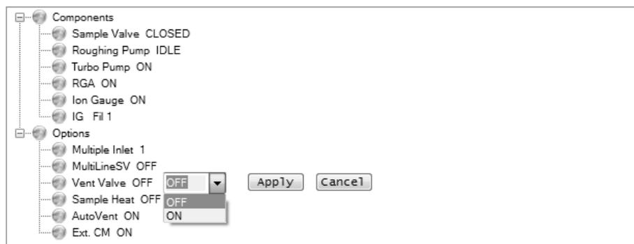
Fig. 2-33. Screenshot of the Vent valve control on the UGA software.
