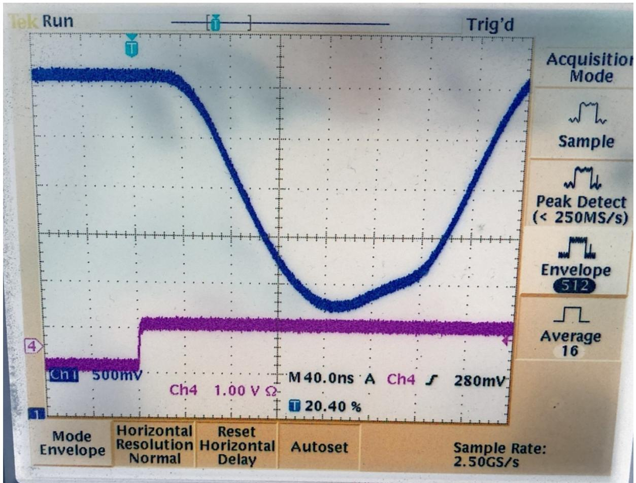
At 40 ns/div, the minor ticks correspond to 8 ns. For both the falling and rising edges, the envelope of the trace can be seen to be less than one minor tick. A reasonable upper bound on the jitter is about  $< 5$  ns jitter.
